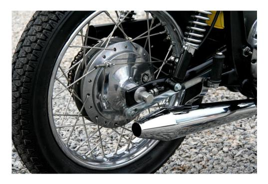
Rear hub reflects more of the extensive polishing efforts I put into the bike. Little "tooter" silencer provides excellent, classic single-cylinder sound. There's a couple more grease fittings. Many of the bike's alloy components required only cleaning and polishing – a testament to decent, original quality, plus suggesting the bike had been well-stored.
