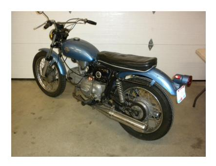
Initial evaluation was quite favorable. The bike had not been run in years, but with quite low mileage, most mechanical parts checked out quite well. The engine was leaking oil from virtually every sealing point, but compression was good, and after a valve job, carb cleaning, and replacement of all gaskets and seals, fired up and ran.
