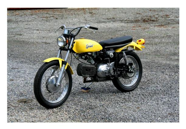
Minus its stock pipes, the Sprint sports some serious ground clearance. Genuine Ceriani forks hold up the front end. The distinctive frame is quite evident in this image. A "spine" type, with the engine suspended below, and held in place with just three mounting bolts! It nonetheless gets the job done, as the design is said have been quite sturdy.
