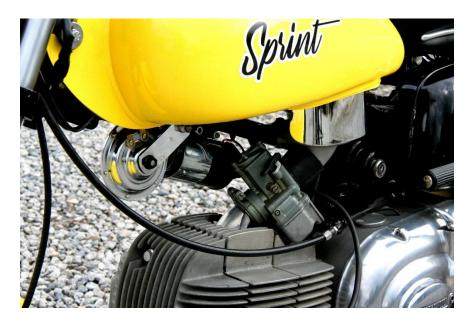
Paper-element air cleaner hangs right out in the breeze, partially hidden behind that chrome cover. Fuel tank is actually dished out a bit to make room for it. Carb is Dellorto, of course.
