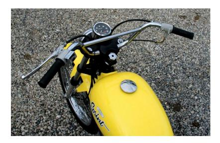
Absence of factory turn signals back in '72 make for quite abbreviated switchgear. Lights are activated at the key switch, so all that's left is a beeper-button, and hi-low beam selector. Anyone who has been around Aermacchis from this era will recognize the control mounts, levers, and big, fat grips.
