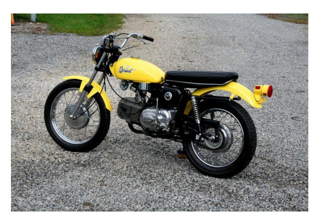
With the single exhaust, left side of the bike looks a bit naked, but quite clean. Very nice replacement seat cover was provided by Mac Motorcycle Seat Covers, which custom made it specifically for this bike. Many original components of the bike were reused after simple basic reconditioning – such as the alloy trim at the base of the seat.
