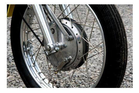
Italian alloys polish up quite nicely. Note the friction-type cable ends. Funky! Grease fitting on brake shoe pivot is a nice touch. Remember, in the European market, these motorcycles were intended to serve as reliable, durable, daily transportation.
